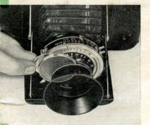
Press the mount on to the front of the lens, keeping the slot at the top. To insert the filter—hold the tag between the thumb and first finger, then place the filter in the slot and press it lightly until it has passed the spring clips (Fig. 14). The filter is now secured and will not drop or shake out.
